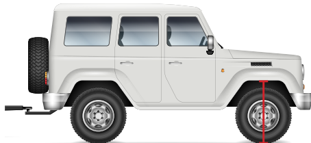
Measure from the ground to the wheel well through the center-line of the axle
